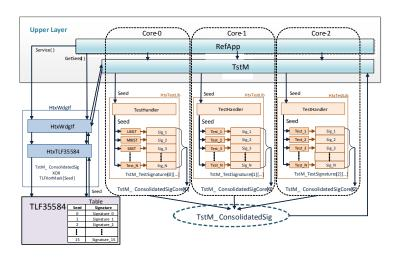
The Safety Watchdog Interface and Signature Monitor are intended to be used both for the AURIX 2G self-test phase and thereafter in the user's application, as in the AURIX TC2xx SafeTLib. This relieves the user from having to create his own TLF35584 servicing system.
